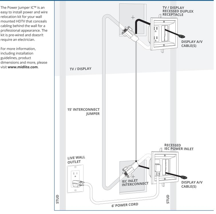
PN: M2PJCTVW15 Conforms to STD 514D and Certified CSA STD 22.2 No. 42.1-00 Electrical Rating: 125 VAC, 15 AMPS, 60 Hz Meets UL 817 & CSA#22.2#21 Interconnect meets UL 2256, 2459 Meets NEC 2014 Article 400.7 (A)(11) Patented with multiple patents pending.
