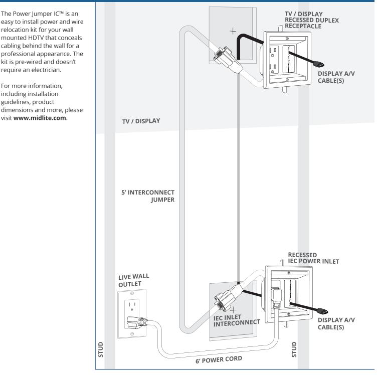
PN: M2PJCTVW5 Conforms to STD 514D and Certified CSA STD 22.2 No. 42.1-00 Electrical Rating: 125 VAC, 15 AMPS, 60 Hz Meets UL 817 & CSA#22.2#21 Interconnect meets UL 2256, 2459 Meets NEC 2014 Article 400.7 (A)(11) Patented with multiple patents pending.
